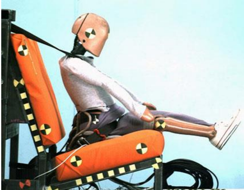
Figure 19. Example of the pelvic belt entering the gap between ATD thigh and pelvis (NT1503).
