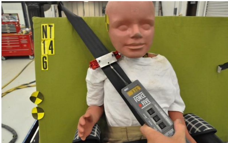
Figure 2. Measurement of resting belt tension with force gauge.
