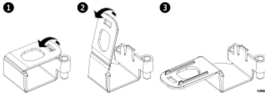
Figure 37 Opening the cable chain lids
