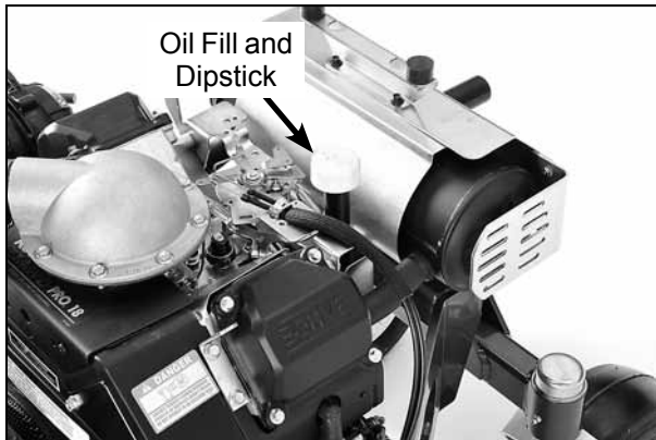
Dipstick and Oil Fill - Model MBK (View from Above Left Side of Tractor)
