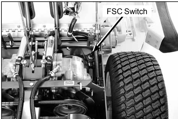
FSC Switch Location
