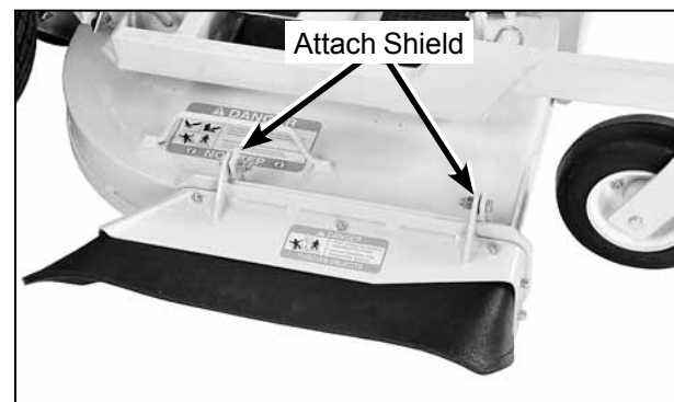
Deck Discharge Shield Installation
