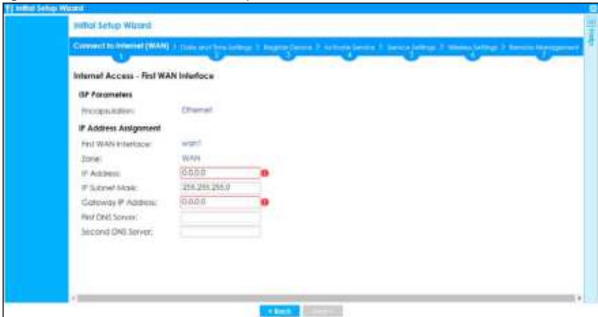
Figure 26 Internet Access: Ethernet Encapsulation
