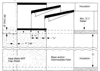
**22.5 Nailable and Lightweight Concrete Decks:** On decks with a slope over  $1\frac{1}{2}$ " per ft (125 mm/m), the roofing felts must be installed parallel to the incline. Nail the end laps of the modified bitumen cap sheet across the width of the sheet on  $8\frac{1}{2}$ " (216 mm) centers. All nails are to be covered by the lap of the next sheet.
