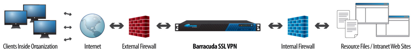
Figure 2.2: Sample layout for DMZ Deployment
