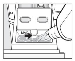
■ Add the fabric conditioner or liquid starch to compartment ⊗. **Do not** exceed the maximum level mark.
