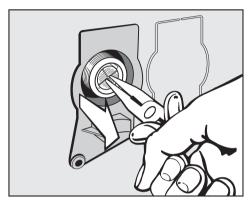
Use water pump pliers to withdraw the plastic filter by the bar (see illustration). Clean, put back and secure.
