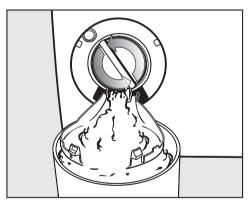
■ Turn the drain filter lid round, until water runs out.
