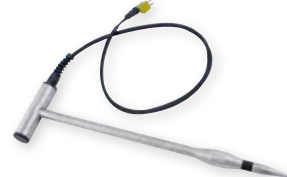
GSF 50TF (110 cm) Art. no. 601312 GSF 50TFK (43 cm) Art. no. 601313 Material moisture insertion probe, with temperature sensor, for measurement up to a depth of 40 cm or 107 cm, incl. 1 m connection cable. Suitable for: wood chips, wood wool, straw, hay, grain, saw dust, etc.
