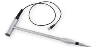
GSF 50 (110 cm) Art. no. 601306 GSF 50K (43 cm) Art. no. 601308 Material moisture insertion probe, (without temperature sensor) for measurement up to a depth of 40 cm or 107 cm, incl. 1 m connection cable. Suitable for: wood chips, wood wool, straw, hay, grain, saw dust, etc.
