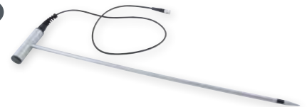
GSF 50TF (110 cm) Art. no. 601312 GSF 50TFK (43 cm) Art. no. 601313 Material moisture insertion probe, with temperature sensor, for measurement up to a depth of 40 cm or 107 cm, incl. 1 m connection cable. Suitable for: wood chips, wood wool, straw, hay, grain, saw dust, etc.
