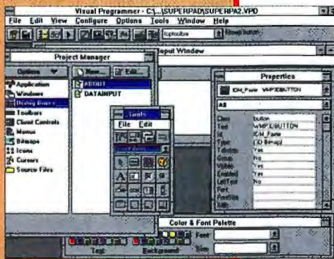
The major new feature in Watcom's latest C/C++ is the addition of visual programming tools.
