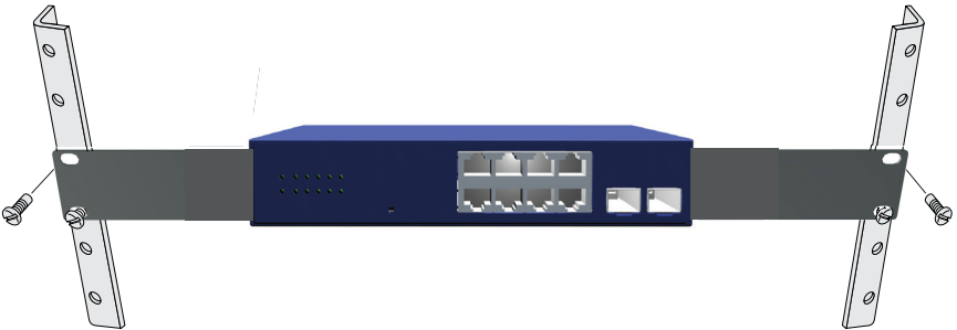
Figure 14: Installing the Switch in a Rack
