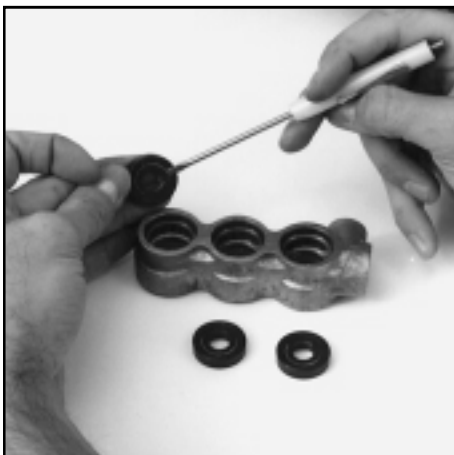
Installation of Lo-Pressure Seals
