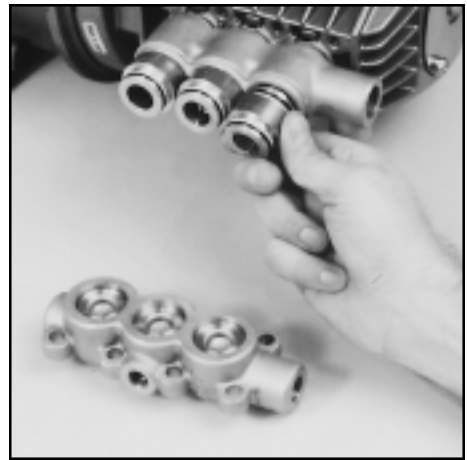
Removal of Adapter from Inlet Manifold
