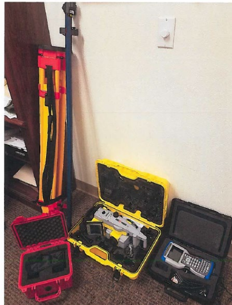
La Paz County Sheriff's Office Total Station measuring device
