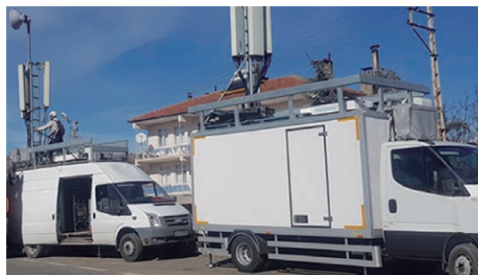
Huawei's network assurance team in Turkey assisting customers set up emergency base stations
