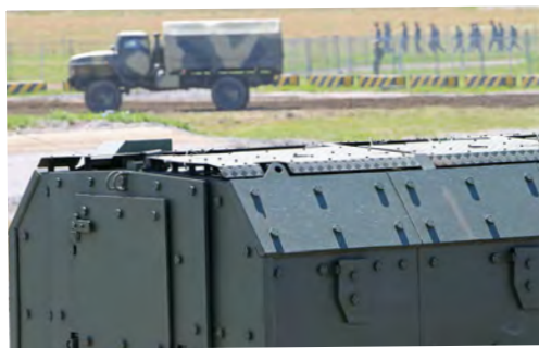
Above: The rear fighting compartment, fitted with applique combination armour.
