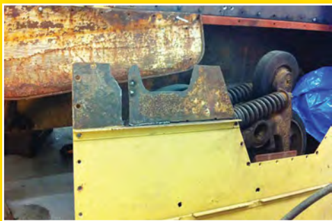
A piece of original armour removed from the bulkhead was incorporated into the rebuilt glacis plate.
