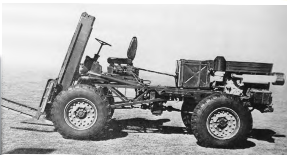
The robust lightweight Eager Beaver forklift truck designed to be air portable and work in forward stores areas. A Perkins 78bhp engine delivered power to all four wheels each fitted with 11X20 Michelin XL tyres. Along with its material handling capabilities the Beaver could tow loads up to 5-tons.
