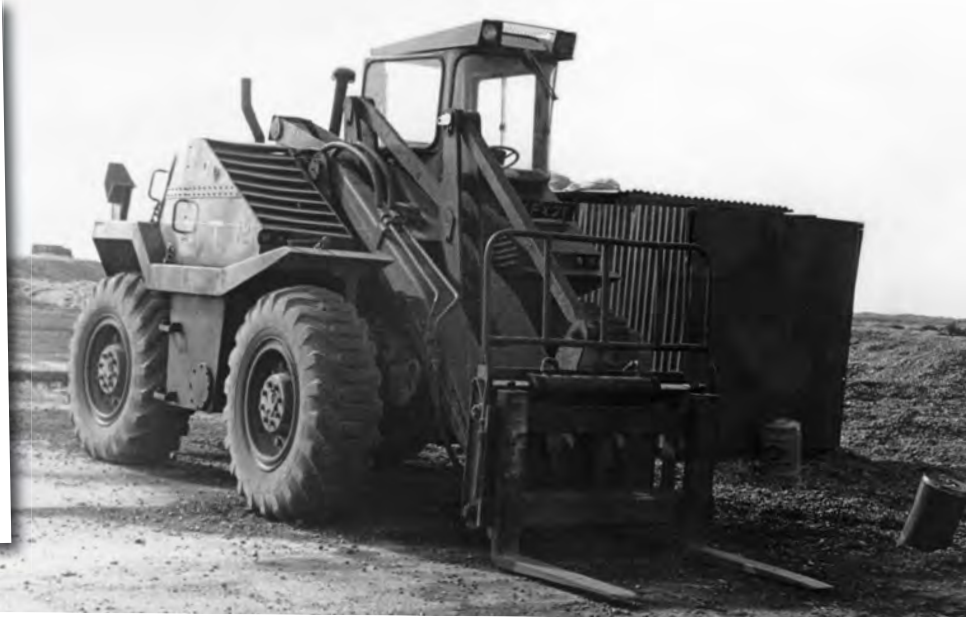
The Muir Hill B 5000 multi-role loader with a fitted backhoe photographed at the Lydd ranges in the 1970s when the Maidstone based engineers were building and repairing some of the roads.
