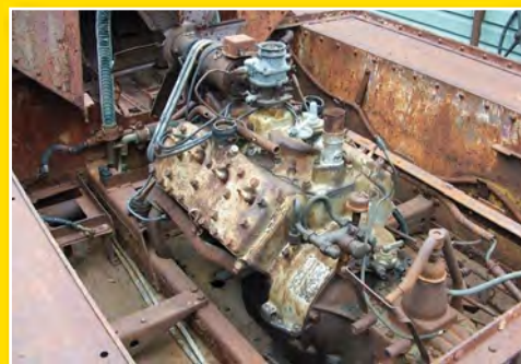
A Ford flathead V8 came with the project but it wasn't the original and probably came from a Ford truck or Mercury saloon.
