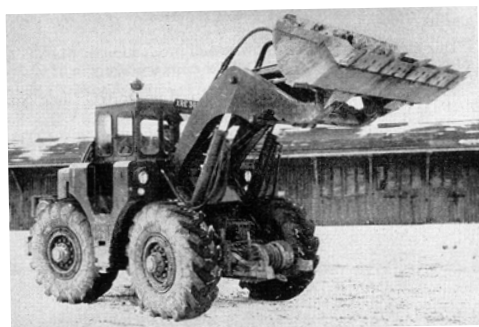
Not the best of images but one that shows the compact design of the early 1950s Marshall Gainsborough front loader.
