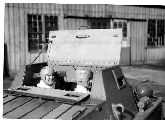
This view of the crew in the CTL-1 tank shows how vulnerable they would have been driving head first into the water. Even reversing would have been risky.
