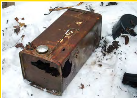
Although past saving, some components such as the fuel tank could be used as patterns.
