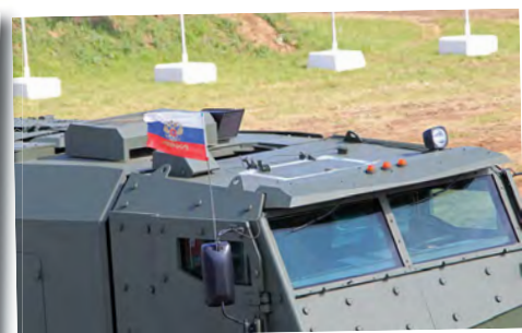
The KamAZ-63968 is also protected from overhead attack from buildings. Two air conditioning systems are installed on the vehicle, one for the cab and the other for the fighting compartment.
