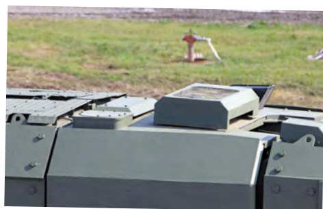
The KamAZ-63968 is also protected from overhead attack from buildings. Two air conditioning systems are installed on the vehicle, one for the cab and the other for the fighting compartment.
