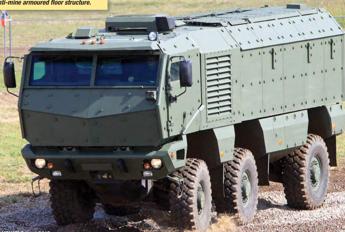
Below: The KamAZ-63968 has a relatively high centre of gravity due to its anti-mine armoured floor structure.
