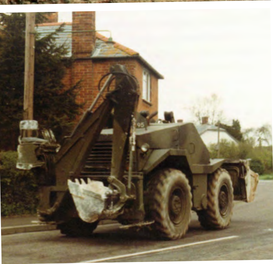
This image shows the backhoe fitted to the Muir Hill 5000. The machine is travelling through Tilshead during Operation Tiger Head on the 3 April 1980. It is unusual to see the machine in operation with the cab removed.
