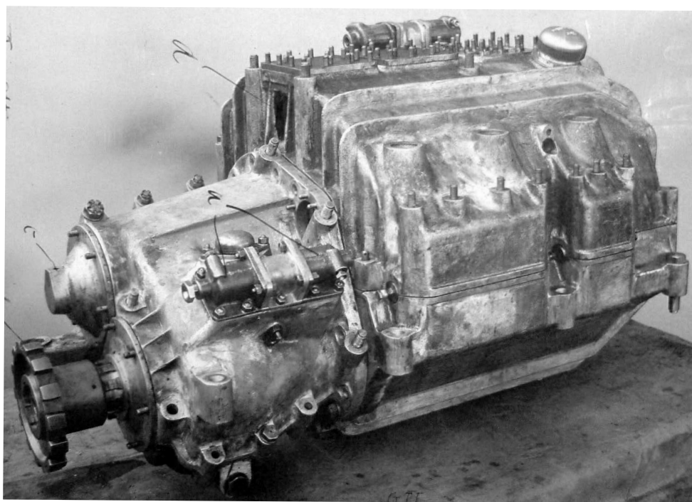
The aluminium housings of the GT I's transmission were loosely assembled for trial purposes. Hydraulic cylinders on the smaller case in the foreground shifted the two-speed gearbox giving the tank a choice of overall ratios.
