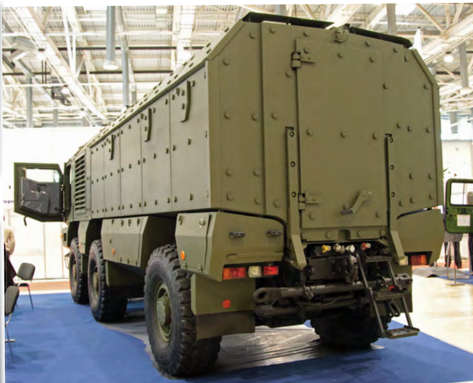
This version of the KamAZ-63968 has a drop down rear ramp incorporating a conventional access door.
