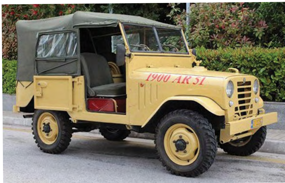
Although no serving military AR51 ever carried that lettering on its bonnet, this picture shows the excellent access from the rear-hinged doors and the petrol tank mounted under the passenger's seat. (Coys)
