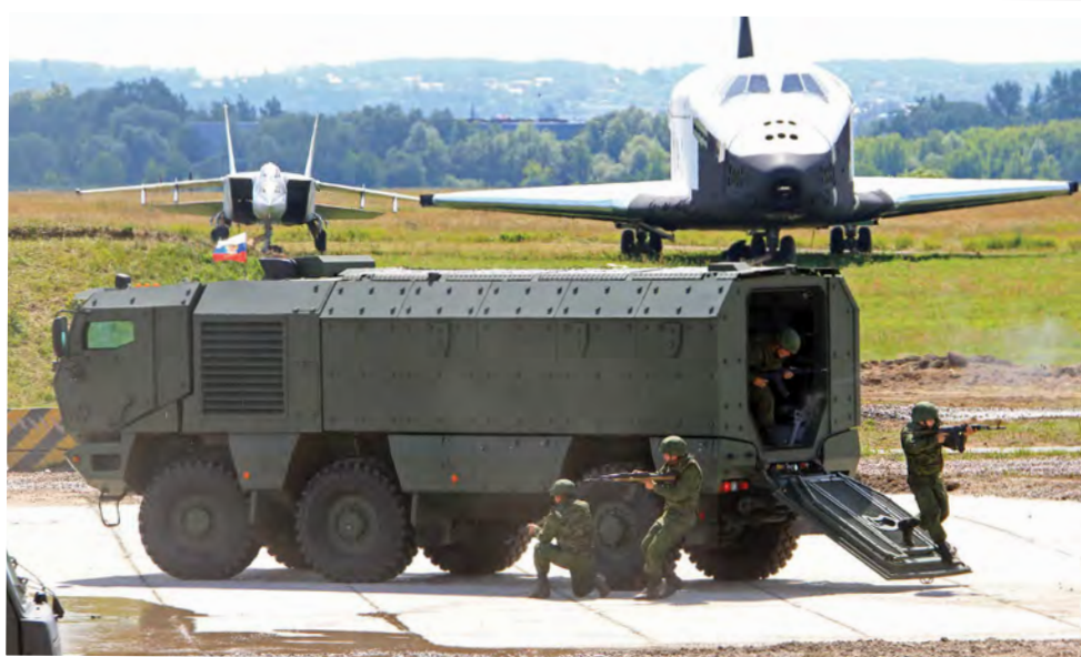
In combat situations, the full infantry section egress the vehicle via the hydraulically operated rear launch ramp, which also incorporates a conventional hatch.
