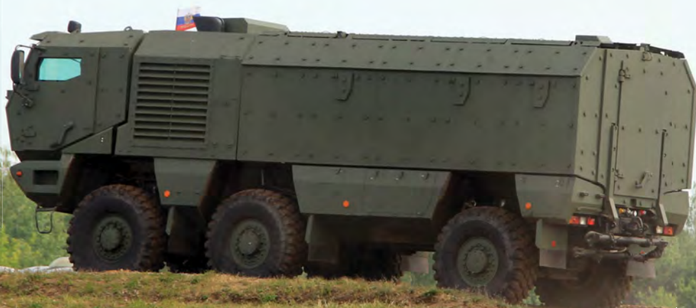
In combat situations, the full infantry section egress the vehicle via the hydraulically operated rear launch ramp, which also incorporates a conventional hatch.
