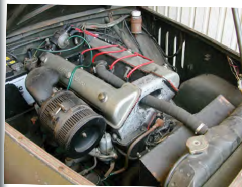
Multi-cam engines are common in modern SUVs, but the DOHC Alfa Romeo engine looks out of place in the Matta. (Unknown copyright)
