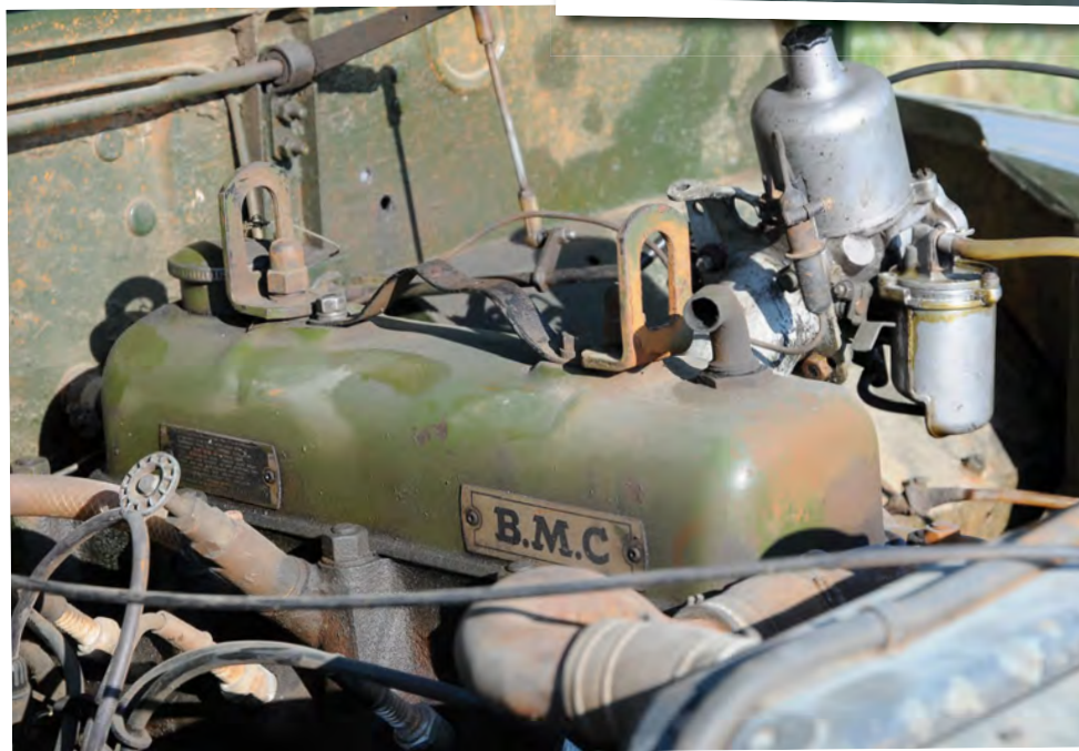
Mechanically, the original 2199cc 70bhp engine was spot on – although Dermot's swapped the original Zenith carb for an SU.
