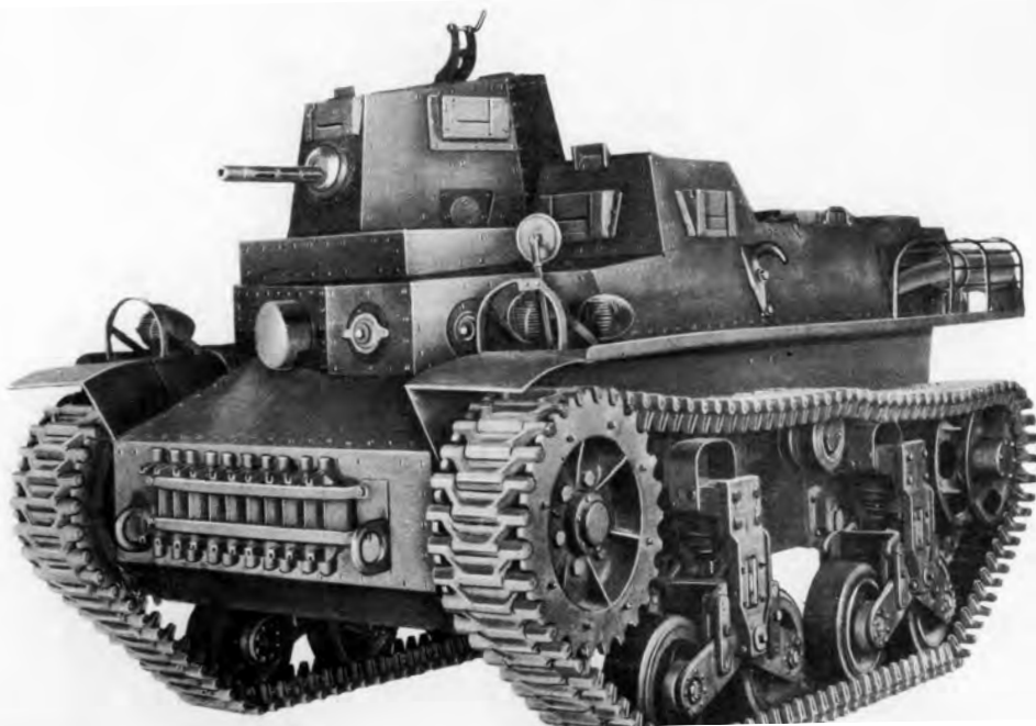
The Marmon-Herrington CTLS-4TAY, or light tank T16 in American service. Note the adoption of vertical volute spring suspension and separate link track.
