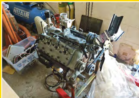
The 99T model 100bhp Ford V8 after a full rebuild.
