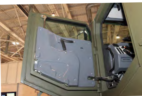
The powered cab doors feature combination armour and armoured glass.
