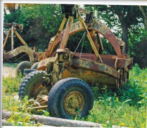
Above and left: The British-built Onions towed scraper here in civilian livery but identical to those supplied to the army. The cable control for the box can be clearly observed in these images of a 8cu yd scraper.
