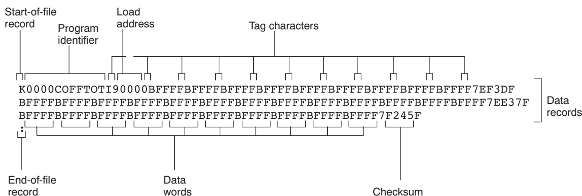
Figure 12-12. TI-Tagged Object Format
