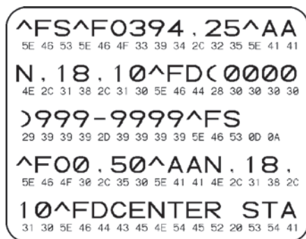
Figure 16 • Communications Diagnostics Test Printout
