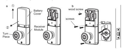
c. Insert 4 (AA) 1.5V alkaline batteries and put the battery cover back to the receiver module.
