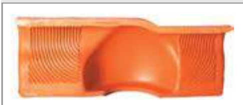
Sectional view of typical insulator cover showing arrangement of ribs. Ribs are engineered to grip the serrations on its corresponding line hose, regardless of angle.
