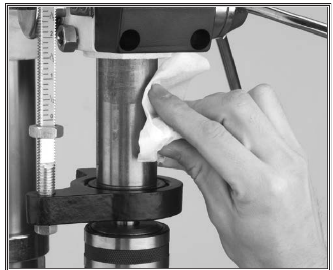
Figure 25. Clean and oil quill shaft.
