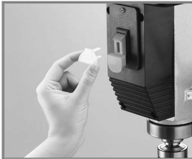
Figure 3. Remove switch safety key when not in use.
