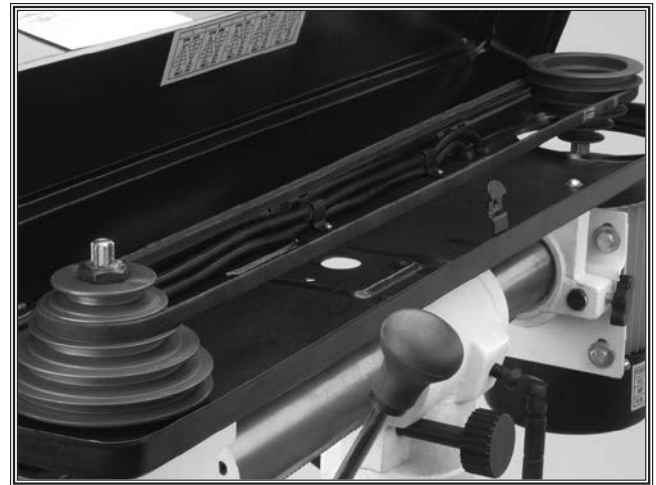
Figure 19. Open belt safety cover.
