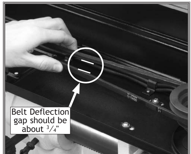
Figure 21. Measuring belt deflection.
