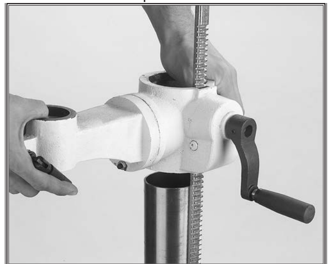
Figure 11. Installing rack and table bracket.
