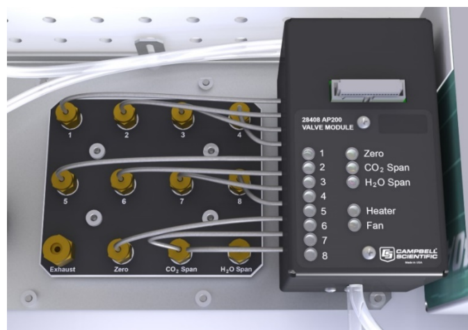
FIGURE 4-21. Valve module and Swagelok® feedthrough fittings on bottom of AP200 enclosure
