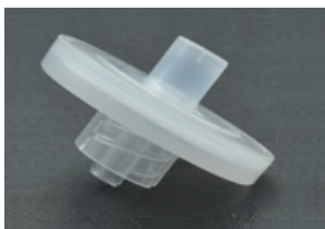
FIGURE 4-12. Syringe filter of current AP200 intake assembly
