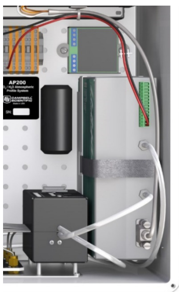
FIGURE 4-4. The IRGA installed in the AP200 system enclosure
