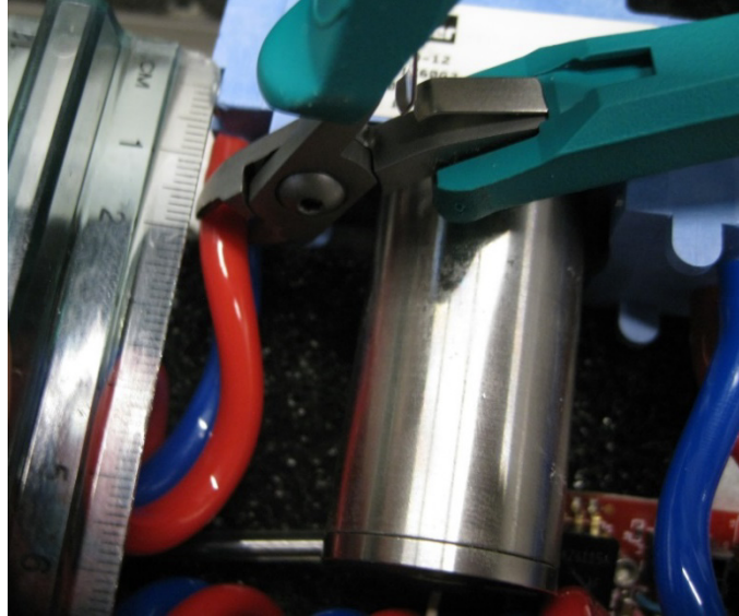
FIGURE J-6. Location of cuts to remove pump assembly from tubing
