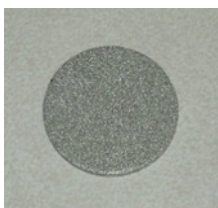
FIGURE 4-13. Disk filter of early AP200 intake assembly
