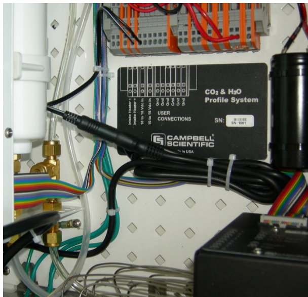
FIGURE G-5. Power adapter output cable plugged into cable extension
