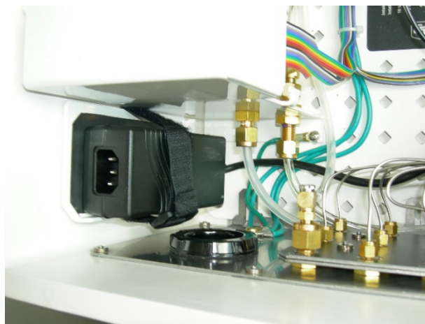
FIGURE 4-8. AC/DC power adapter kit installed in AP200
