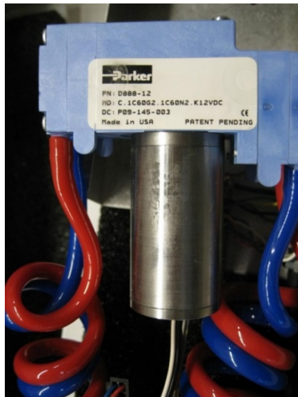
FIGURE J-7. Inlet and outlet tubing reconnected to pump
