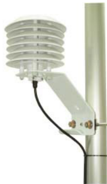
FIGURE 4-10. 107-L temperature probe mounted with radiation shield
