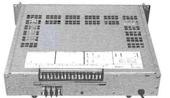
TYPICAL REAR VIEW SHOWING ACCESSIBLE TERMINAL BLOCKS WITH SIMPLIFIED CONNECTION GUIDE AND PROVISIONS FOR VIX REMOTE SIGNALING
