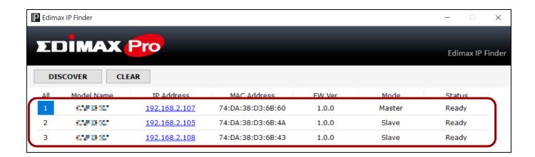
7. Click the IP address of the master access point to go into the web user interface.
