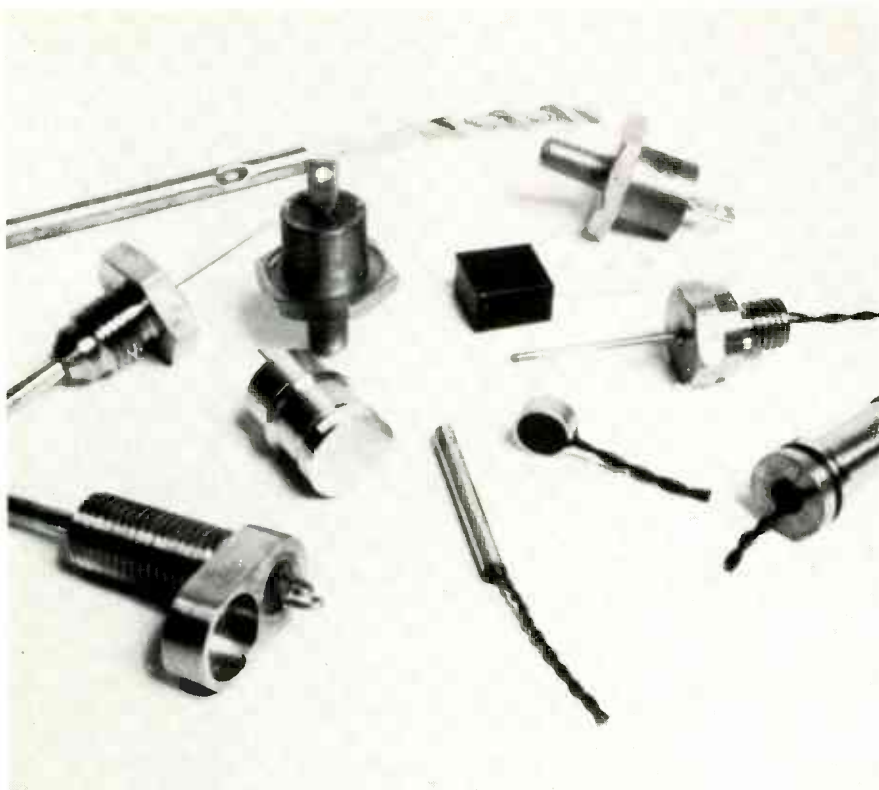
THERMISTORS ARE HOUSED in a wide variety of enclosures for different applications. Among the enclosures shown here are ones for air, water, and surface temperature measurement.
