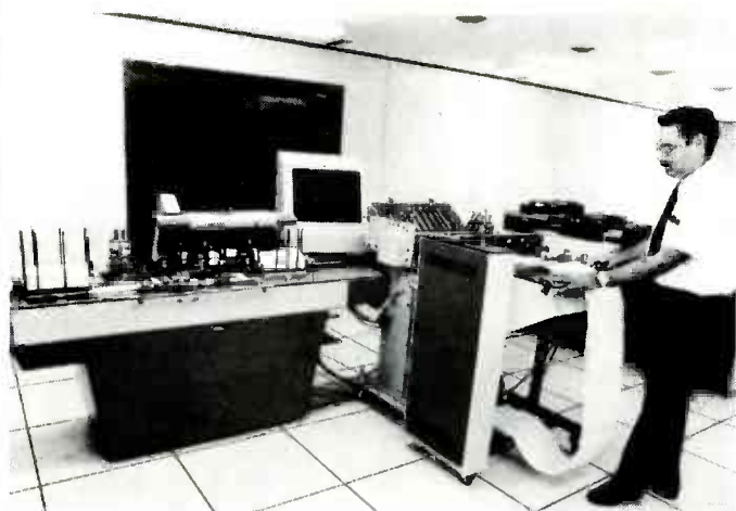
E-COM EQUIPMENT UNDER TEST at the RCA Government Communications Systems, Camden, NJ. (RCA supplied the equipment for the new system, on a $31-million contract.) The system accepts inputs from a customer's computer-generated magnetic tape or from a computer via private telecommunications carriers and transmits it to the electronic center designated by the customer, where it is printed, trimmed, folded, placed in envelopes, and delivered by first-class mail.
