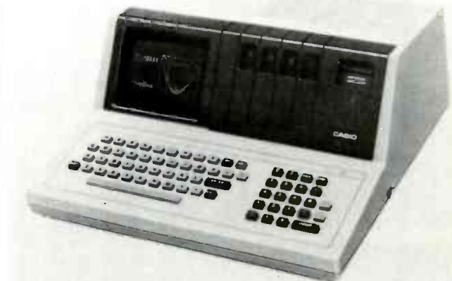
THE CASIO FX-9000P personal computer. The basic unit comes with a 4K RAM, a 5.5-inch built-in CRT, very extensive high-resolution graphics, and powerful mathematical functions for scientific, engineering and statistical operations.
