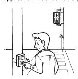
When the pedestrian pushbutton is pressed for a traffic signal, the signal light changes from red to green after a delay.
