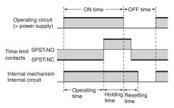
The resetting time of the Timer is the period of time during which all the internal components including the contacts, pointer, and the circuit components, such as the capacitor, of the Timer are reset.
