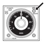
The operating mode selector is in the upper-right corner on the H3CR-A.
