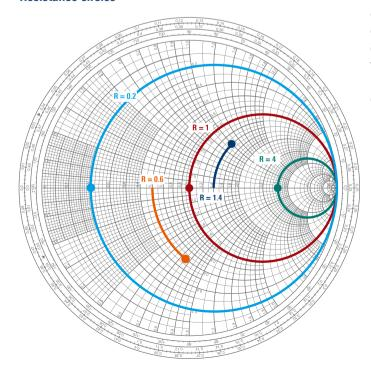
For a traditional Smith chart, the resistance rises from 0 (leftmost side of the chart) to infinite (rightmost side of the chart). The upper half of the chart shows positive values of jX, thus designating an inductive behavior of the impedance, while in the lower half of the chart those values are negative and the behavior is capacitive. Please be aware that the Smith chart is normalized to the reference impedance (50  $\Omega$  or 75  $\Omega$ ) depending on the equipment used.
