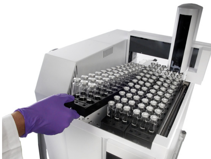
Figure 16 Removing vial racks from the tray assembly (111-Vial Model)
