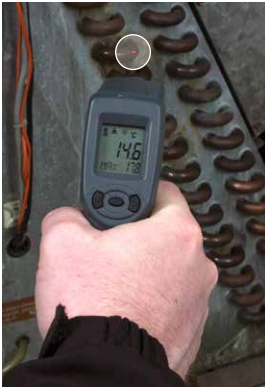
IR thermometer: temperature measurement in one spot
