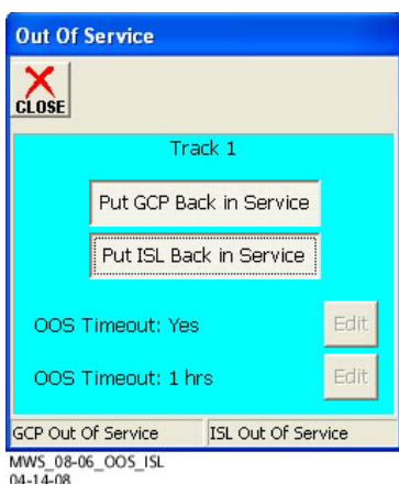
Figure 43: Return Track to Service Window
