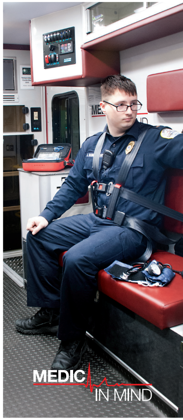
Medic in Mind layout with 6 point restraint and single seating position – cabinets fore and aft of seat keep equipment within arm's reach
