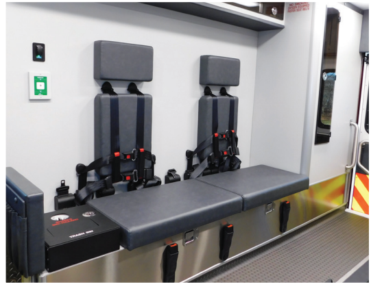
Full length squad bench with multiple seating positions utilizing 6 point harnesses
