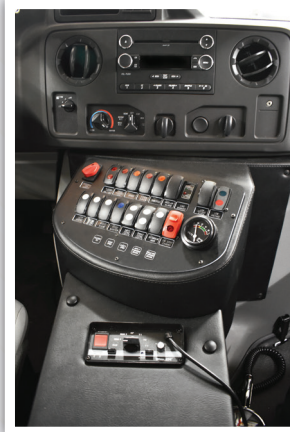
Conventional electrical system with elliptical console design
