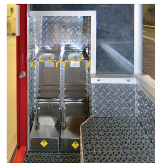
Intermediate side entrance door step with recessed "D" bottle storage.
