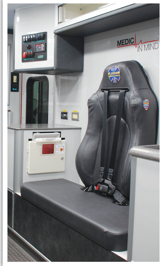
Optional Medic in Mind with Valor Backrest 4 point restraint with 4 retractors and single release buckle
