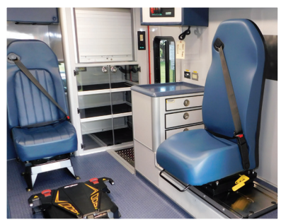
Side facing captain chair on sliding track for additional access to patient
