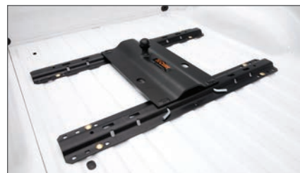
C Using pre-existing 5th wheel base rails
