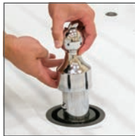
Step 2 - Drop the ball into OEM puck system hole
