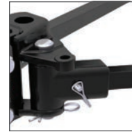
Pin-style spring bars improve strength
