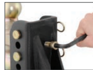
Built-in anti-rattle prevents shaking
