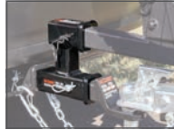
45792 provides two receiver tubes
