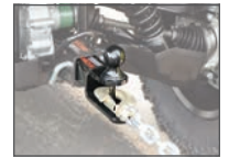
Clevis pin accepts hook or strap for straight-line pull
