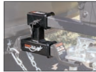
45792 provides two receiver tubes
