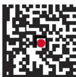
Figure 3-9 DS36X8-DP and DS36X8-DPA Aiming Pattern
