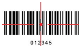
Figure 3-7 DS36X8-HD and DS36X8-HP Aiming Pattern
