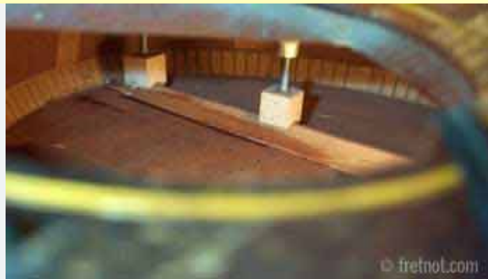
"Jacks" are often used to glue loose back braces
