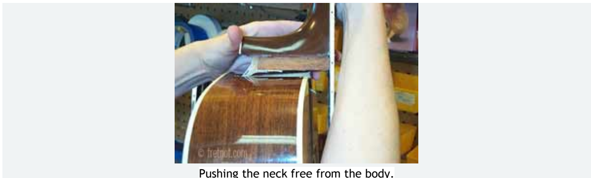
Pushing the neck free from the body.
