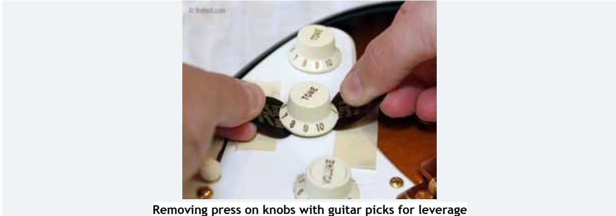
Removing press on knobs with guitar picks for leverage
