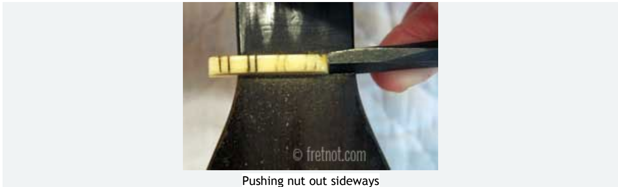
Pushing nut out sideways
