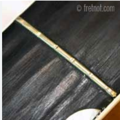
Strings wear grooves in the fret's crown.
