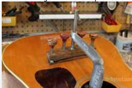
Regluing loose bridge
