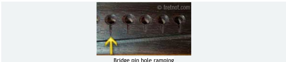
Bridge pin hole ramping
