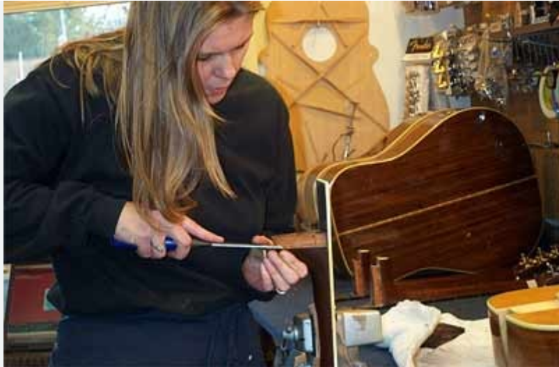
A new taper of the heel's sides will increase the neck angle.
