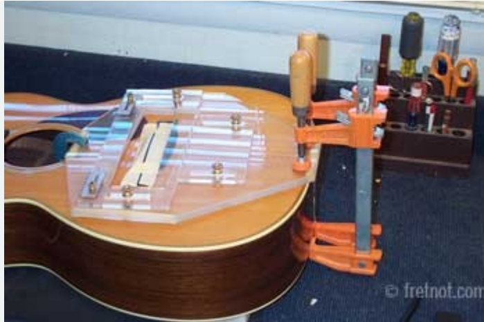
A bridge slotting jig serves as a guide for my laminate trimmer.
