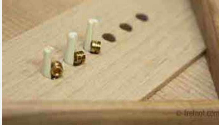
String ends seated firmly against maple bridge plate.
