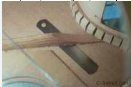
A thin feeler gauge will slide under a loose brace.
