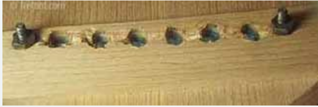
Gibson guitar bridge plate showing signs of wear.
