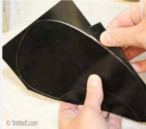
Plastic is scored heavily and snapped free
