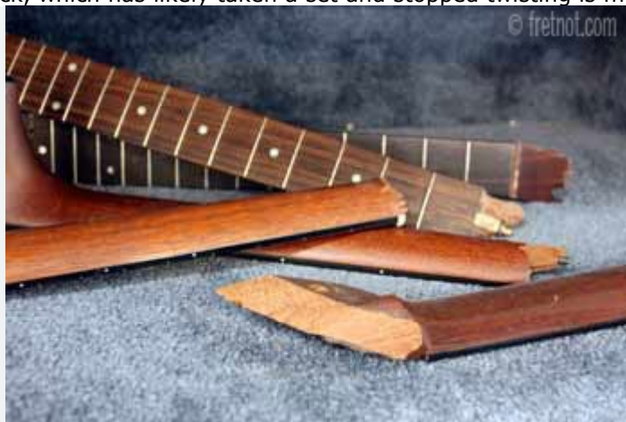
Breaks frequently occur where the peghead meets the neck.
