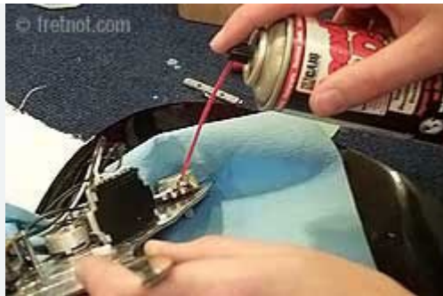
Pots can be cleaned by spraying into the open area of the pot below the soldering lugs.
