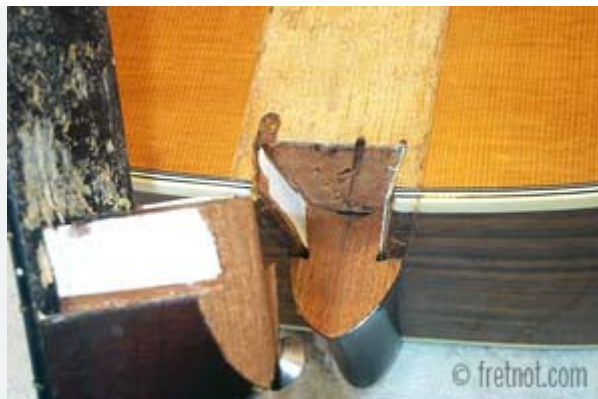
This neck heel fractured after coming loose and being left under tension.
