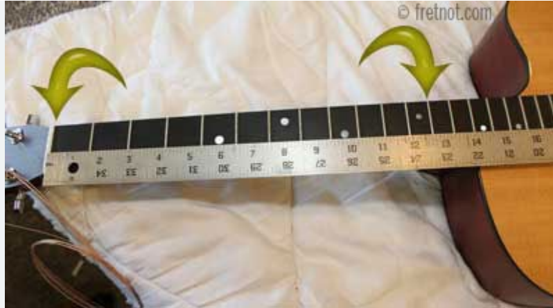
Scale Length can be determined by measuring from the end of the fingerboard, to the center of the 12th fret and doubling it.
