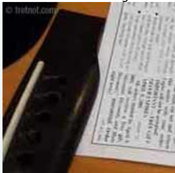
Thin paper slid beneath loose bridge.
