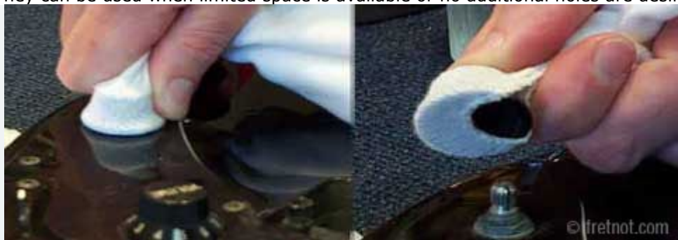
Removing press on knobs with rag
