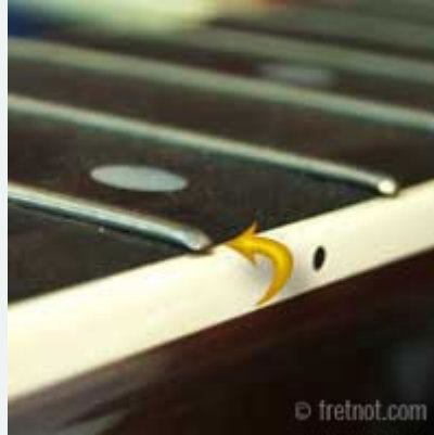
Loose fret ends often catch the treble E string when bending.
