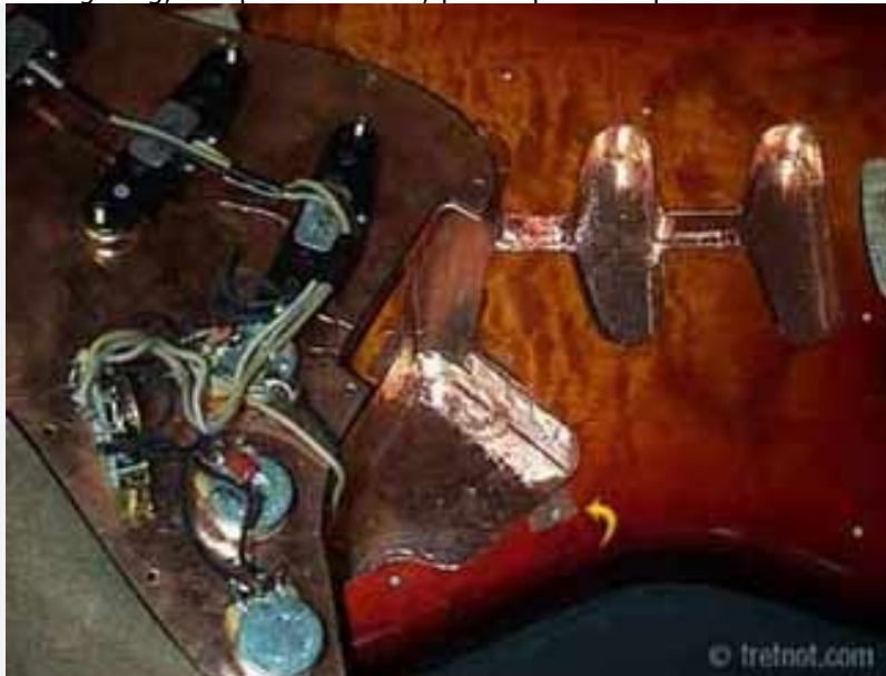
Shielding lines the routed cavity as well as the back of the pickguard. A "tab" is used to complete the connection from cavity to pickguard.
