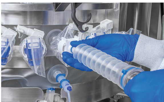
Figure 10. Bioreactor probe assembly.
