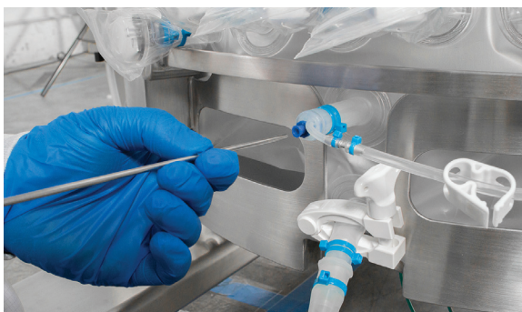
Figure 9. Temperature sample port.
