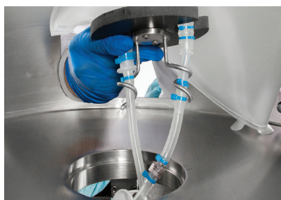
Figure 3. Sparge line support.
