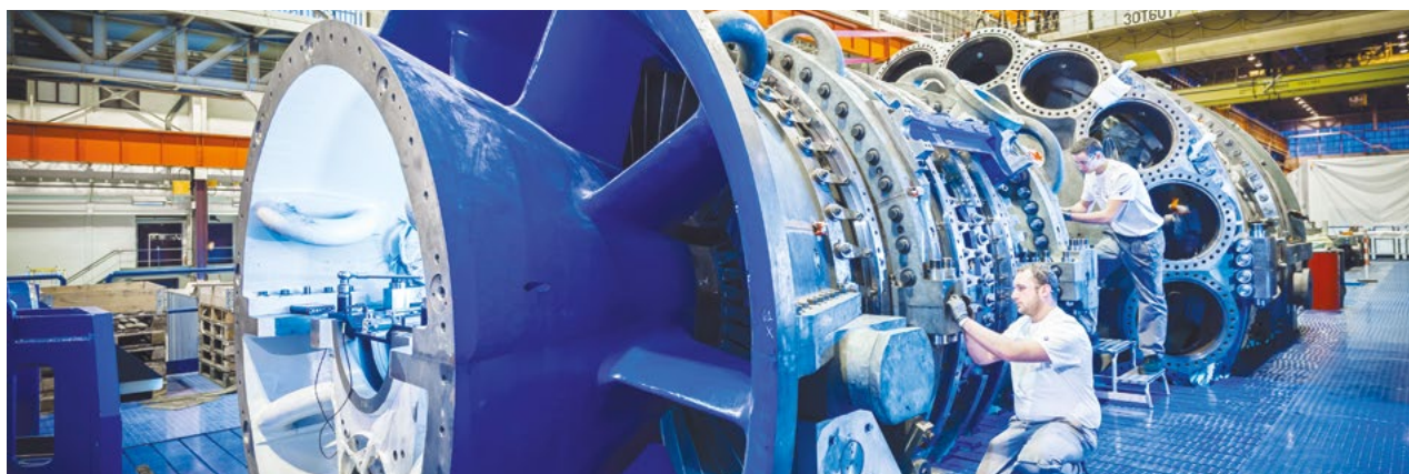
GE's HA gas turbine
