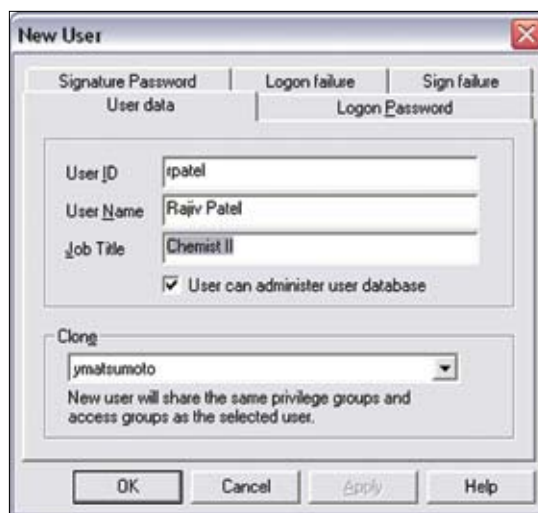
Figure 11. Users are identified by User ID, User Name, and Job Title throughout the software.
