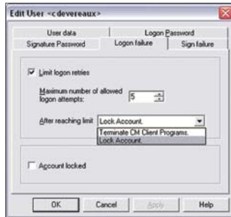
Figure 13. Users can be automatically locked out after a pre-set number of login failures.
