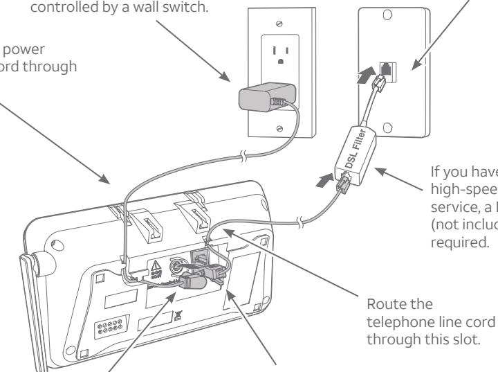
Plug the small end of the telephone base power adapter into the power adapter jack on the back of the telephone base.
