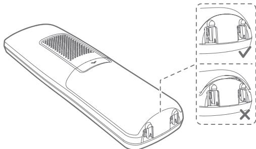
3. Charge the handset by placing it face forward in the telephone base or charger. The **CHARGE** light on the top of the handset is on during charging.
