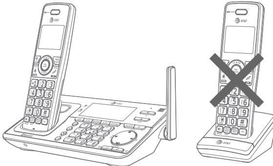
For registration, put the handset on the telephone base, not the handset charger.
