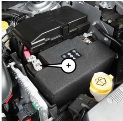
Positive Battery Post
