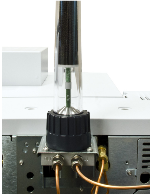
Figure 41. Unscrew the knurled or plastic ring nut
