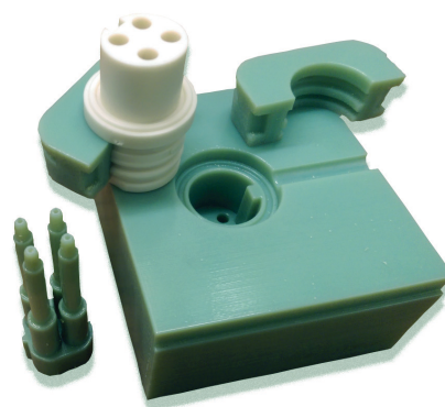
Complex component molded in a 3D printed mold
