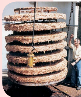
This is what is leftover from 1,000 kilograms of rose petals after extraction.
