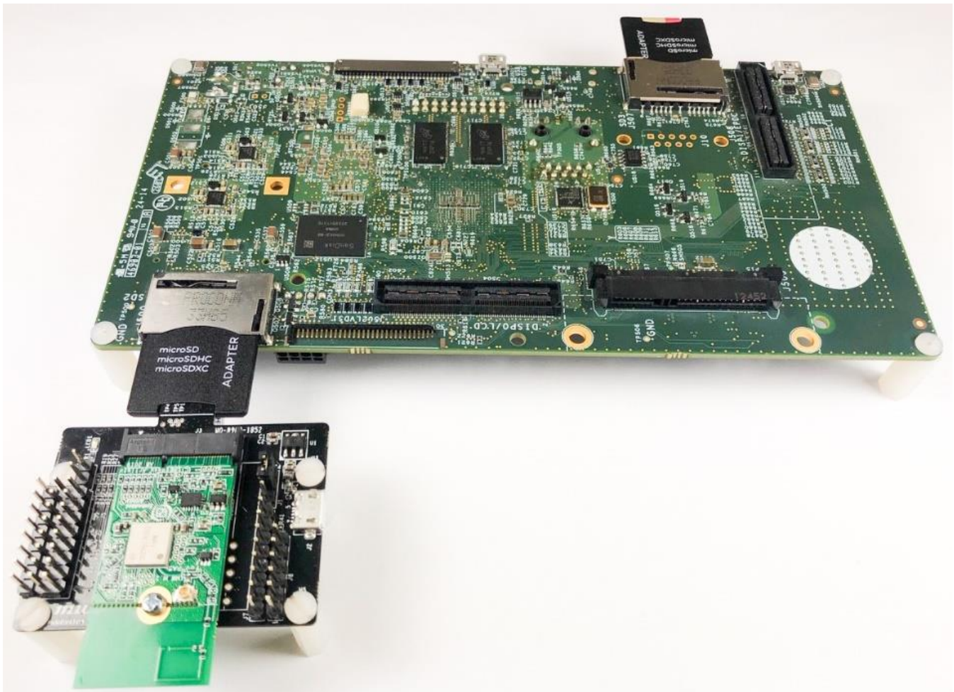
Figure 9: i.MX 6Quad/DualLite SDB (Inverted) with uSD-M.2 Adapter and Type 1MW M.2 EVB
