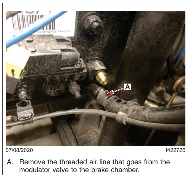
Fig. 7, Removing the Threaded Air Line
