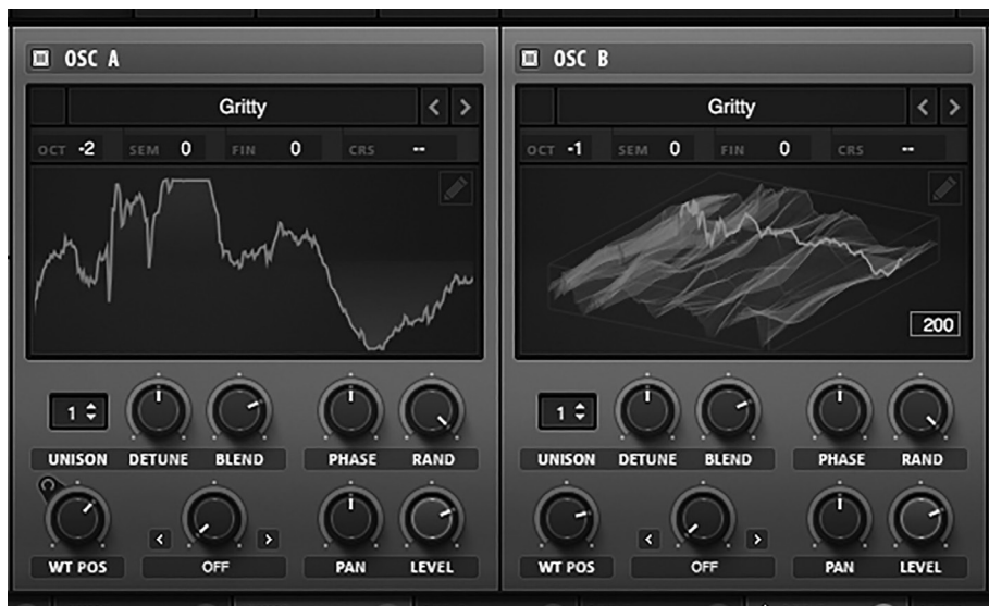
FIGURE 7.8 The gritty wavetables are detuned by octaves, and then you can scan through to find an exciting sound in both
