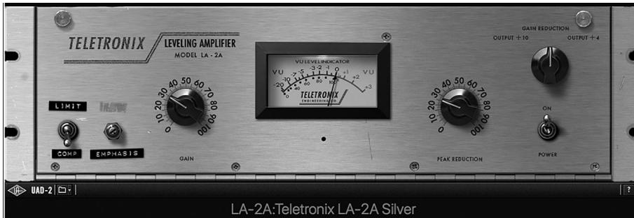
FIGURE 11.11 The LA2A compressor
