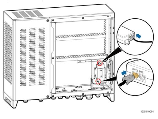
Figure 5-14 Connecting cables to the PoE module
