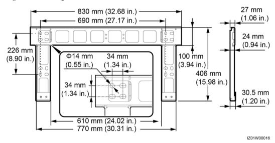
Figure 4-2 Mounting bracket dimensions
