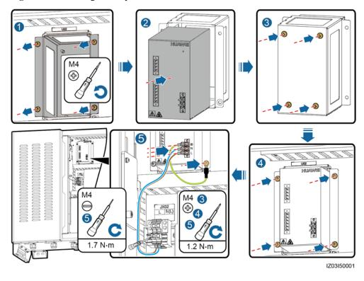
Figure 4-12 Installing a 24 V power module
