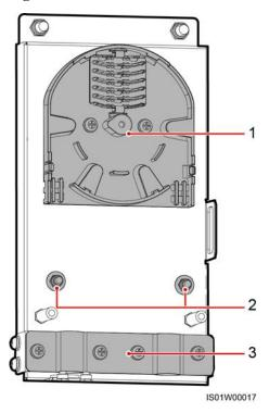
(1) Fiber spool (2) Fixing points for internal steel wires of optical cables (3) Cable clip
