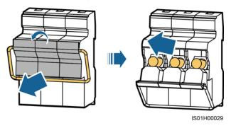
Step 2 Install a new fuse and close the knife fuse switch box.
