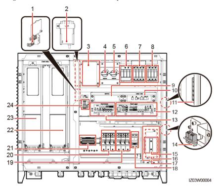
Figure 2-5 SmartACU2000D-D-03 Components
