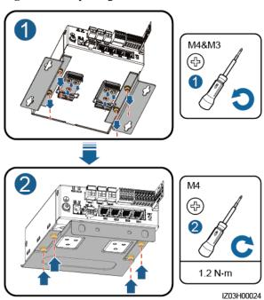
Figure 7-10 Replacing a SmartModule
