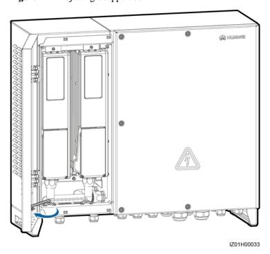
Figure 7-12 Adjusting a support bar
