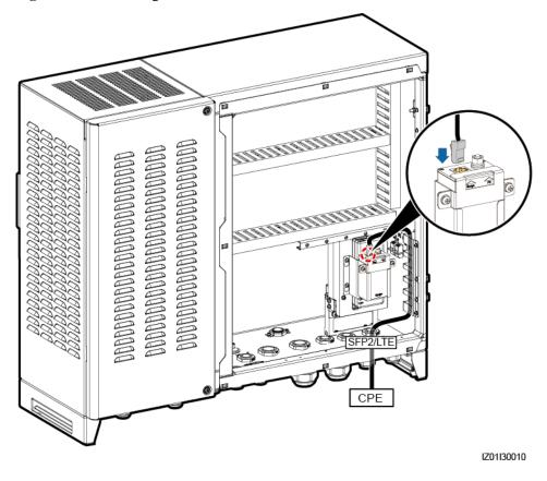
Figure 5-13 Connecting the CPE network cable
