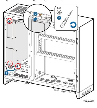
Figure 7-14 Removing a faulty PID module
