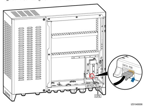
Figure 5-15 Connecting a CPE network cable
