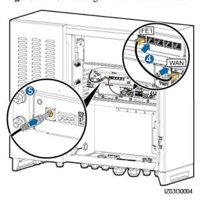
Figure 4-11 Connecting an Ethernet switch cable
