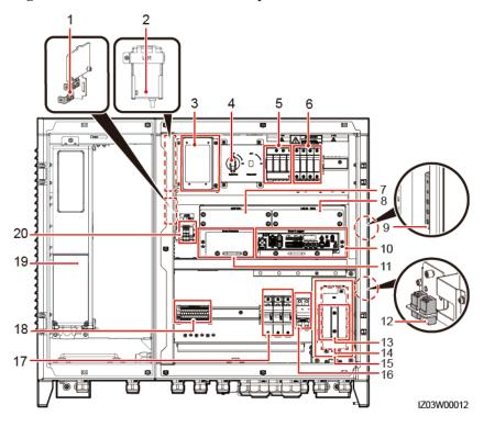
Figure 2-6 SmartACU2000D-D-01 Components
