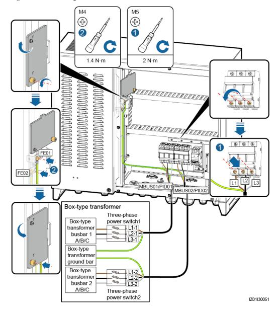
Figure 5-17 Connecting a cable
