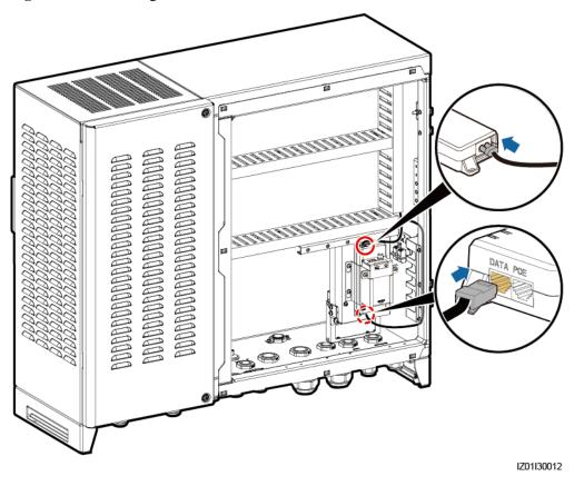
Figure 5-12 Connecting cables to the PoE module
