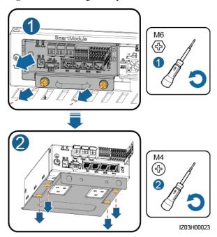
Figure 7-9 Removing a faulty SmartModule
