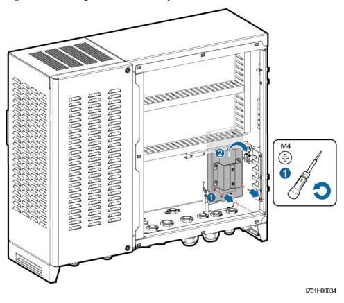
Figure 5-8 Removing external mechanical parts
