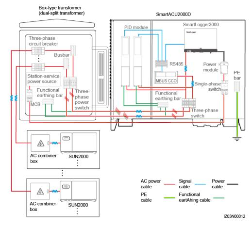
Figure 2-9 MBUS communication mode
