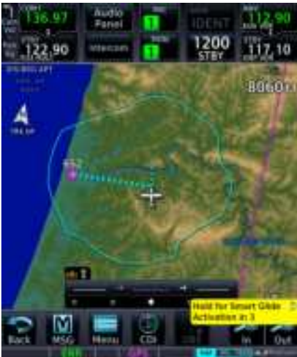
The "Hold for Smart Glide Activation" control label appears near the bottom of the display when you activate the feature using the Direct To key.
