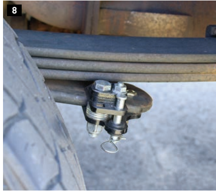
7) A \frac{3}{8} -inch ratchet and extension are used to engage the Quick Disconnect stabilizer. 8) A clip and pin keep it in place in the engaged position.
