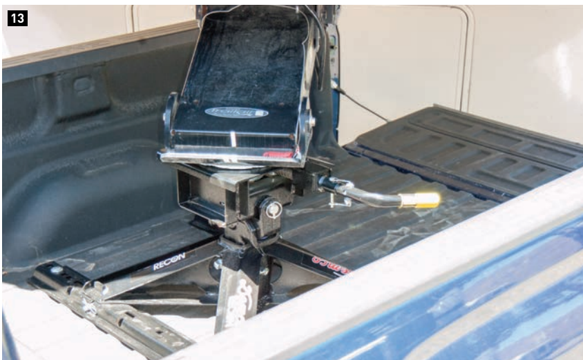
11) Before mounting the hitch head to the saddle assembly, a urethane damper is press-fit into the specified location. 12) The latching handle can be mounted facing front or rear to meet the needs of the owner. 13) The articulating head made it easy to hitch and unhitch on undulating terrain.
