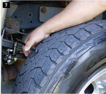
7) A \frac{3}{8} -inch ratchet and extension are used to engage the Quick Disconnect stabilizer. 8) A clip and pin keep it in place in the engaged position.
