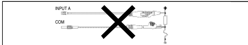
(Incorrect Grounding) Noise Pickup on Unshielded Ground Lead
