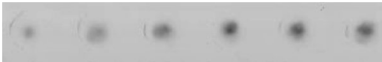
Fig. 25. Representative bombardment showing penetration of 1.6 \mu m gold particles into Parafilm Laboratory Film at (left to right) 100, 200, 300, 400, 500, and 600 psi using the Helios Gene Gun.
