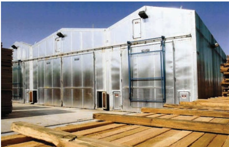
Three American Wood Dryers (two single track and one double track) have a combined drying capacity of 240,000 board feet of lumber.
