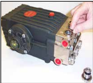
Figure 5-4. Apply Grease and Install Valves
