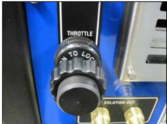
Figure 4-4. Turn Throttle Cable Knob Counterclockwise to Increase
