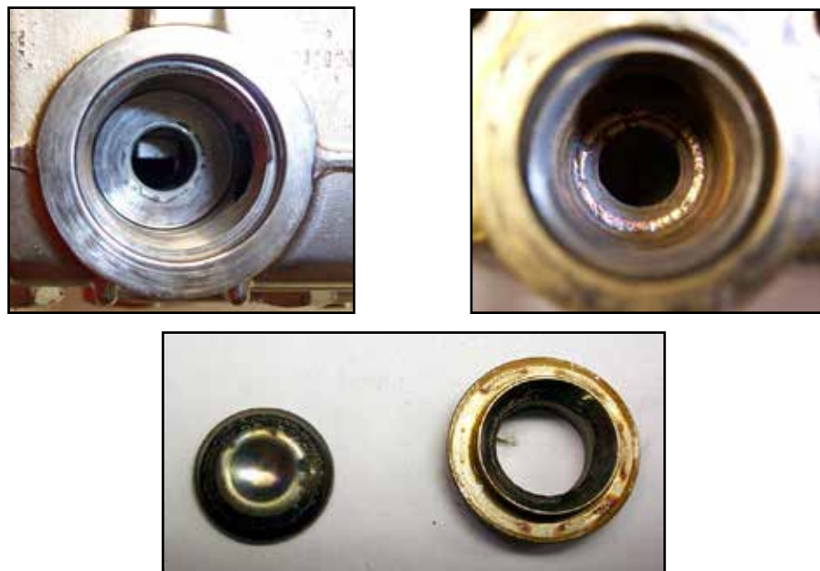
Figure 5-2. Inspect Manifold and Old Valves
