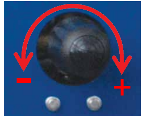
Figure 4-5. Adjust Pressure by Rotating Valve Left (Decrease) or Right (Increase)
